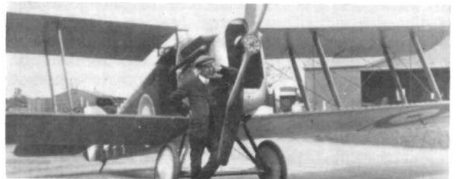
Harry Hawker with the first prototype. This photograph illustrates clearly the shape of the nose radiator.
