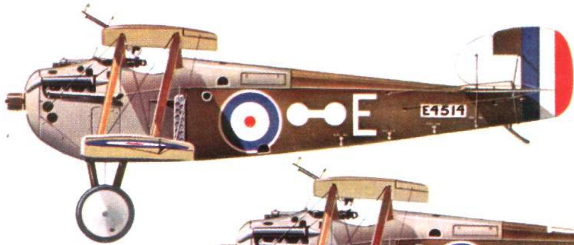
Dolphin E4514, aircraft 'E' of No. 19 Squadron; France 1918. Single (starboard) Lewis gun.
