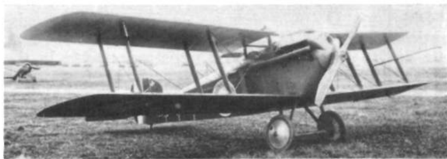
(Above) The first Dolphin II, D3615, with 300 h.p. Hispano-Suiza engine. This photograph shows how the extended exhaust pipes of this version were cranked over the radiator blocks. The presence of a Morane-Saulnier M.S.30E-1 clearly indicates that the photograph was taken in France.
