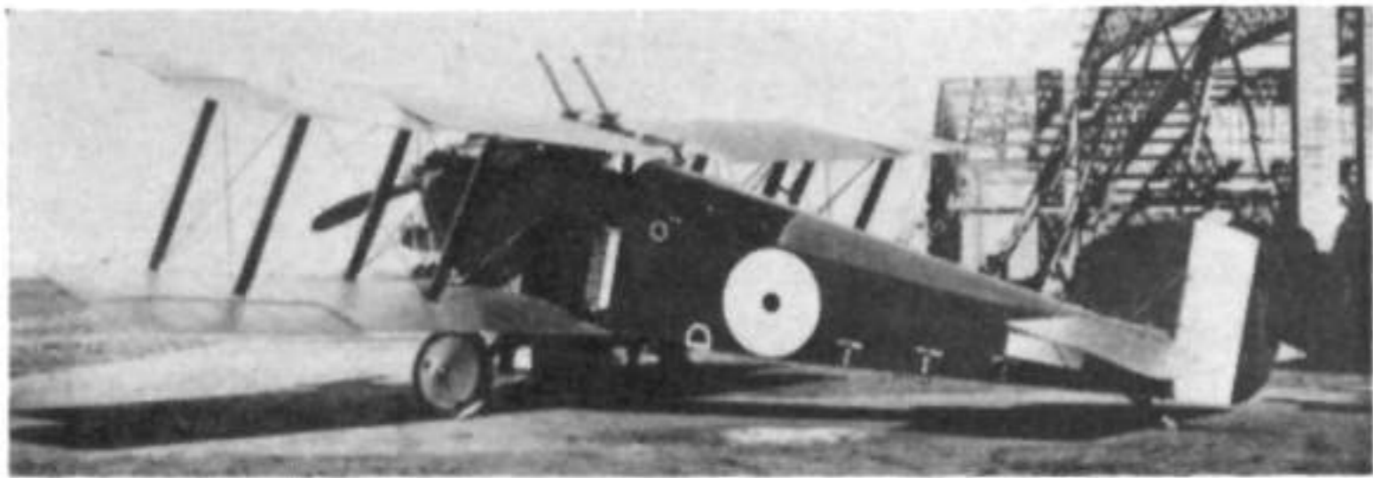
The fourth prototype Dolphin at Martlesham Heath. This aircraft differed from its immediate predecessor in having the top decking behind the cockpit reduced in height; and the small locker in the port side of that decking was moved aft.
