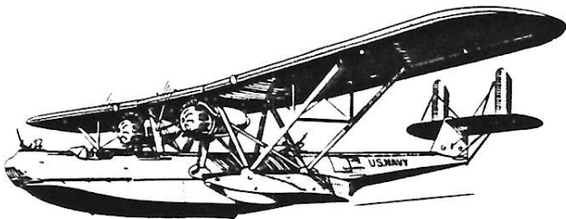
MARTIN P3M-1 Large U.S. Navy patrol bomber. It was produced fitted with amphibious gear.
