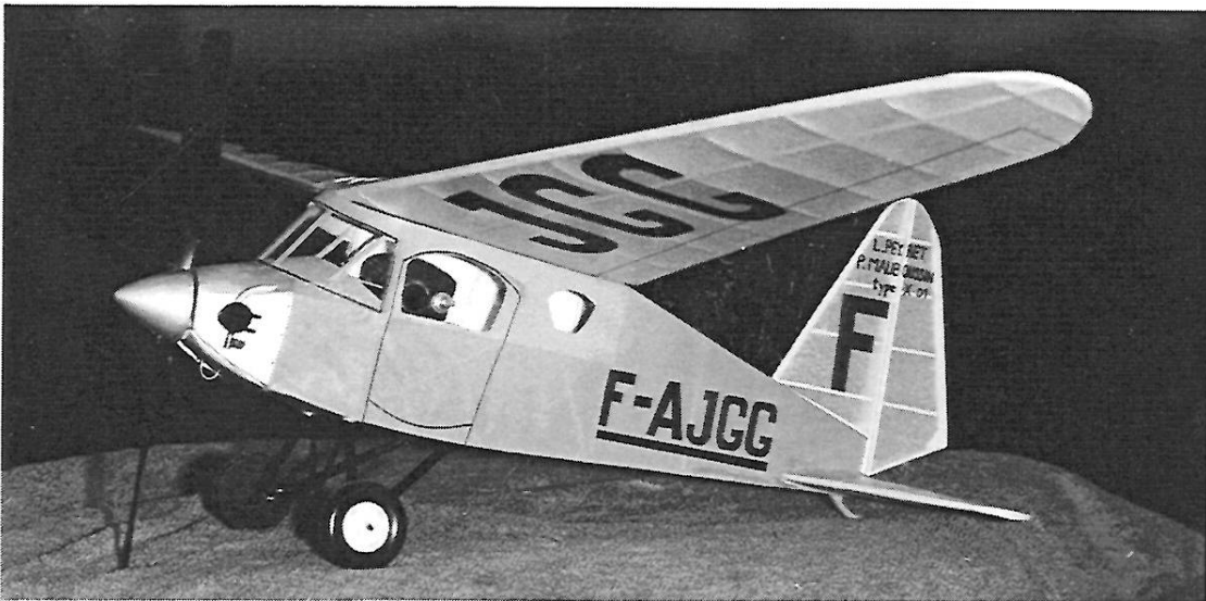
Terry Pittman's Mauboussin P.M. X (or P.M. 10) from an enlarged E. Fillon plan. Almost identical to the Mauboussin P.M. 4 shown elsewhere in this issue. The P.M. X set a number of distance and endurance records in France in 1929 and 1930. Model is powered by a Brown A-23 CO2 motor with a sleek streak prop. Tricky to trim with all that vertical stab, short moments, and high aspect wing, but has done 90+ seconds outdoors.
