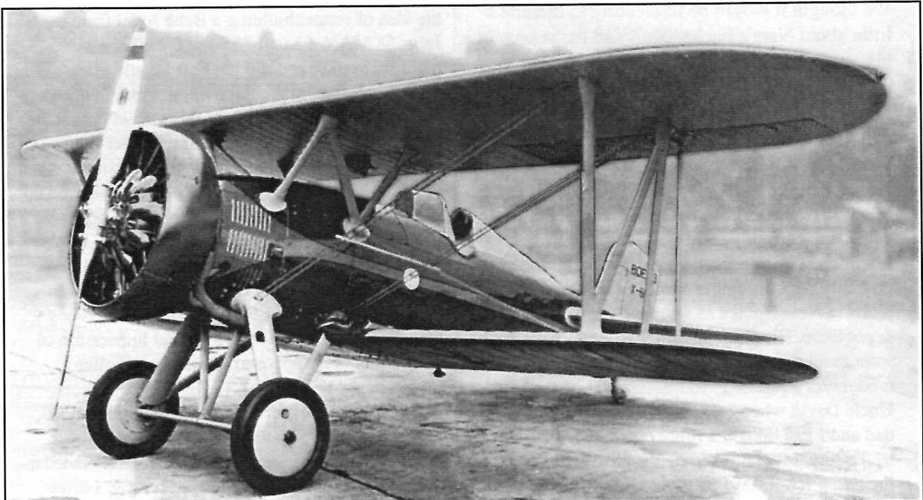
Original form of the Model 218, which introduced a new monocoque metal fuselage structure to the established F4B/P-12 line and served as the prototype for both the P-12E and the F4B-3. (Boeing Photo)
