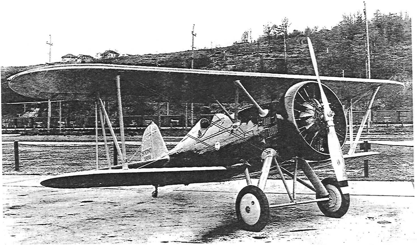
R-1340D and XP-925A with R-1340E. Used to test new features, including introduction of metal monocoque fuselage to the P-12/F4B line. (Photo - The Boeing Co., 4157B, courtesy of Harl Brackin)
