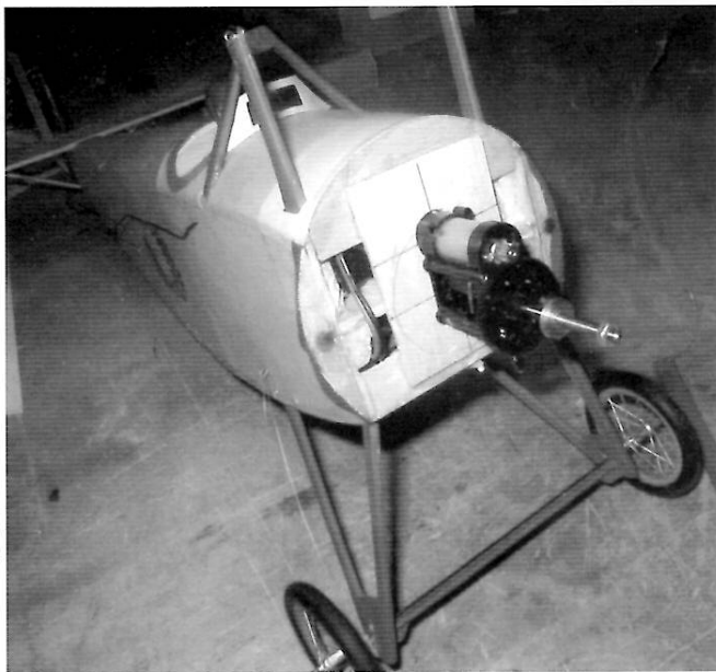
Here the cowl has been removed to show the GWS-A motor installation. The round dots on the cheek cowls are the magnets that hold the cowl on. The dummy motor had not yet been installed. It is held in by magnets in a similar manner.
