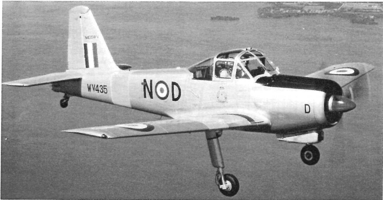
It seems a pity that such a modern looking aircraft as the Provost T1 should have fixed undercarriage.
