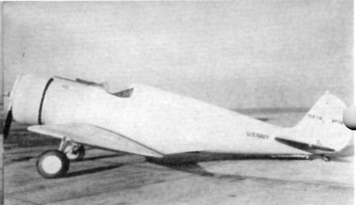
Latest improvements included NACA long-cowl and flaps, but Navy reverted to the open cockpit. An even draw for progress.
