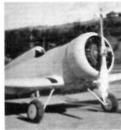
For carrier operations better visibility "necessitated" an open cockpit.
