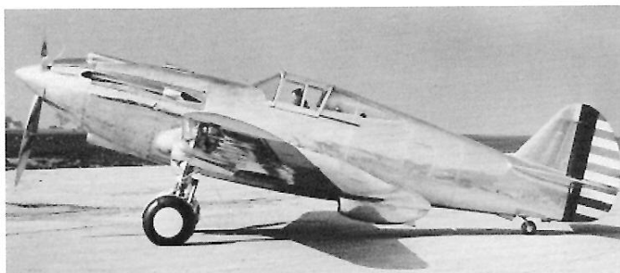
THE XP-40 CONVERTED FROM A P-36 WITH THE ORIGINAL AFT RADIATOR INSTALLATION, THE SUBJECT OF THIS ISSUE.
