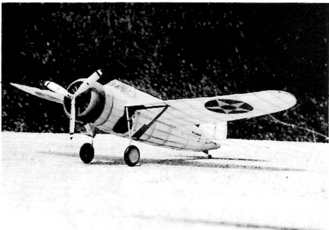
Landing gear on real Brewster folded into both wing and fuselage. Careful duplication of this complex gear impresses scale judges.
