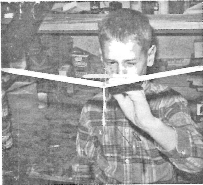
An important part of building a flying model is checking out the alignment of flying surfaces. Should not be crooked — no warps!
