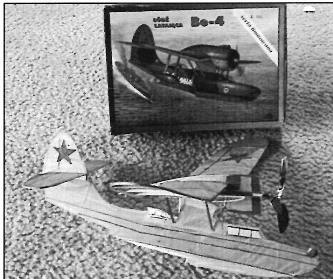
Bruce's first version of the BE-4. Note motor tube running under wing; V.2 (as presented on plan) is substantially modified.
