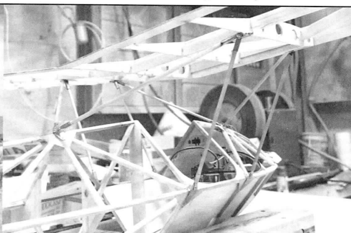
Close up of the cabane struts of Dave's Abbot-Baynes SCUD 1 glider. Tricky little beastie. Though the model is being built for FAC Scale Hi-Start glider, Dave is installing rudder and elevator R/C to allow for flying on small fields.
