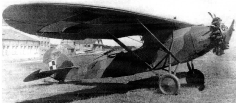
(above) This looks to be an R-XIIIA. The rear fuselage appears flat; an observers cockpit and machine gun have been fitted.
