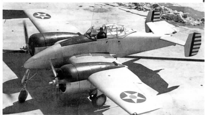
The XP-50, a further development of the XF5F-1 with accomodations for more armament, turbo charged engines, and tricycle landing gear.
