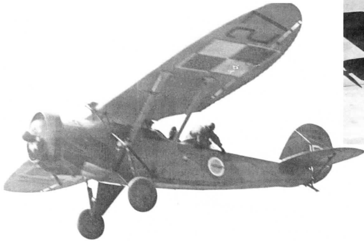
Fly-by view of an R-XIII-D. Note the observers cockpit, LG fairings, Townend cowl, and fairing that runs under the bottom of the nose.
