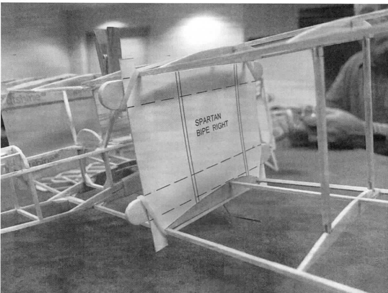
Close-up of a typical wing-incidence jig that Stew Meyers uses for his bipes. Takes the guesswork out of it!
