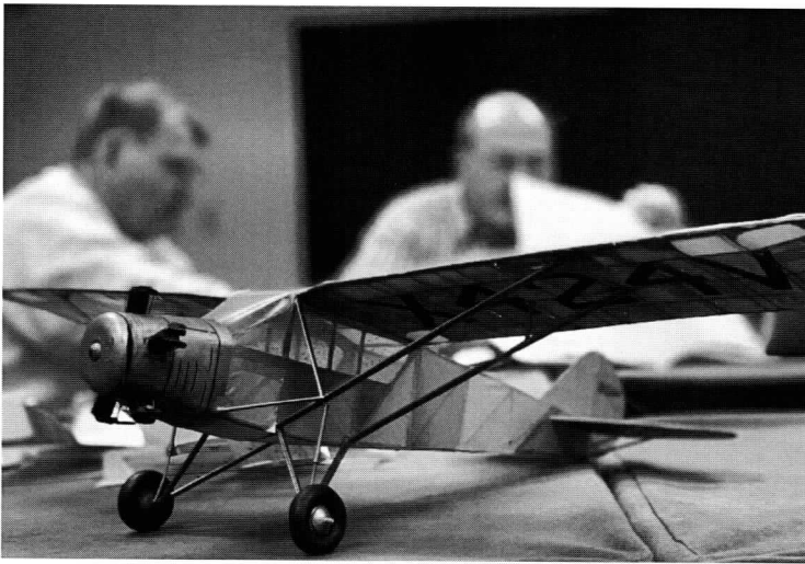
Glen Simpers brought in one of Bill Bell's old models, a Lincoln APK5 from Hurst Bowers' plans. Glen has been using it as a testbed to test the efficacy of different airfoils ...
