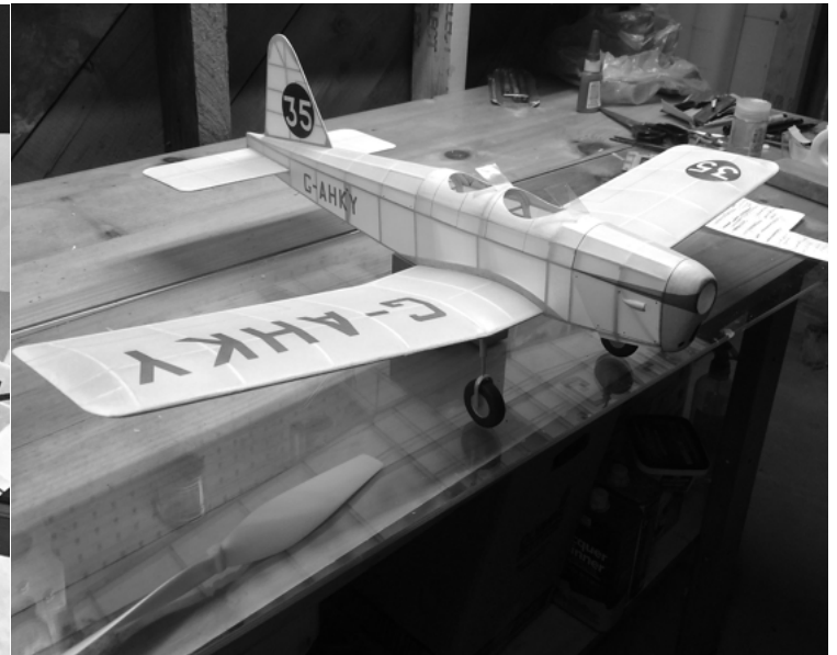
Tom's Miles, done up in King's Cup livery. At 24" wingspan, Tom says they're both coming in at about 28g for a very attractive wing loading of .25g/sq.in.
