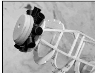
The simple finished engine in place, with the nose plug fitted.
