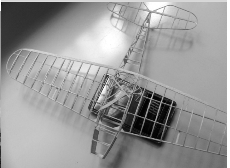
Enrique Maltz is building a peanut version of Tom Hallman's Babcock Taubman design (above). That scale reads 1.8g....!
