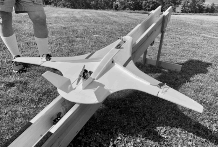
David Eames' nifty catapult launch NAV-72. Dave calls this a "blended wing body" design, which is based on an airliner concept he's worked on at Rolls Royce
