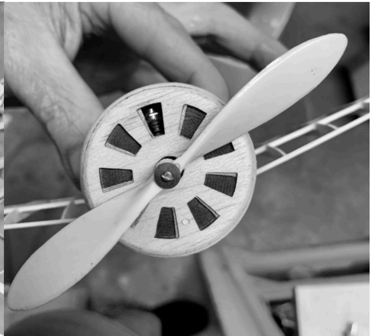
The business end of the I-16. Removing the prop allows the cowl front to be removed, for adjusting the rpms. The motor is mounted via soft copper wire clinches to a plywood plate. That plate is then fitted into a blocked-up recess in the cowl assembly and held in position by rare earth magnets.
