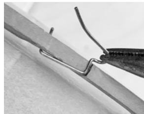
Tow hook in position on the skid; several wraps of 1/16" rubber will hold it in position
