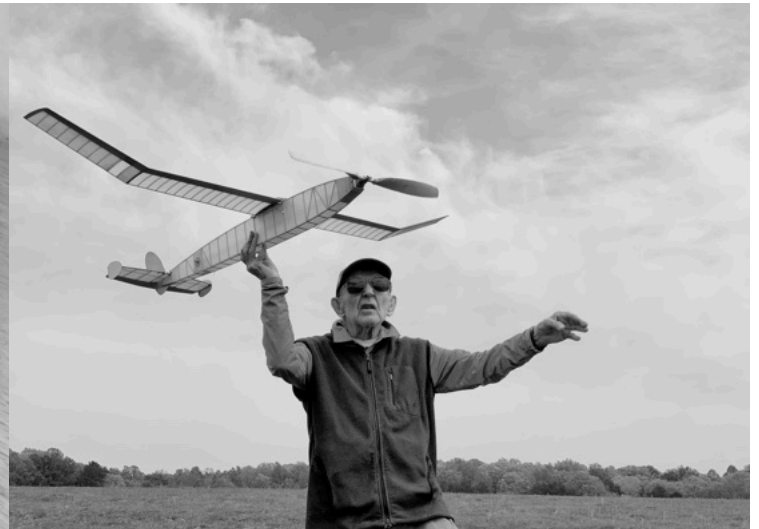
Don Srull gives his Cluge Special the heave ho. A mishmash of parts from different aircraft, Don used it to test out a spectacular balsa and composite wing that he got his hands on. Carl Hampton shows us the wing (below). Check out that undercamber! The wing is razor-thin and stiff as a board. As you might expect, the Cluge is a slow and graceful flier.
