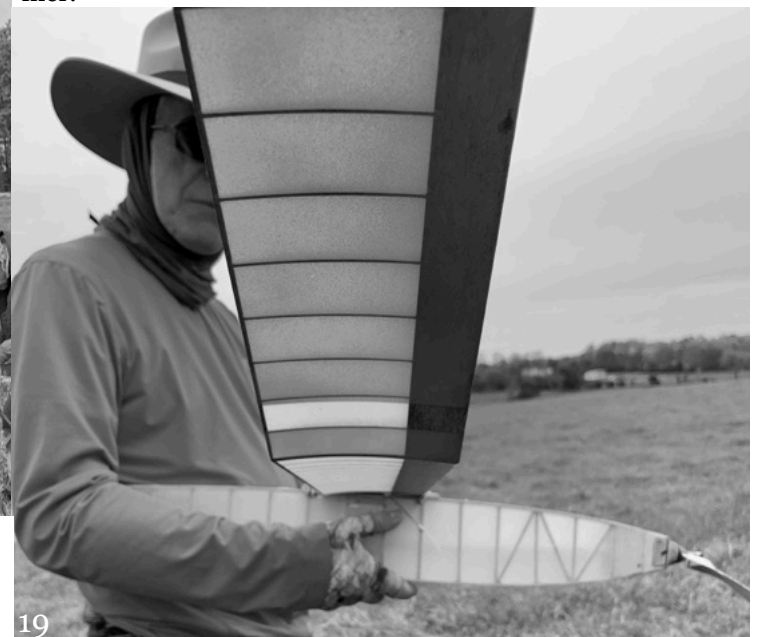
Don Srull gives his Cluge Special the heave ho. A mishmash of parts from different aircraft, Don used it to test out a spectacular balsa and composite wing that he got his hands on. Carl Hampton shows us the wing (below). Check out that undercamber! The wing is razor-thin and stiff as a board. As you might expect, the Cluge is a slow and graceful flier.
