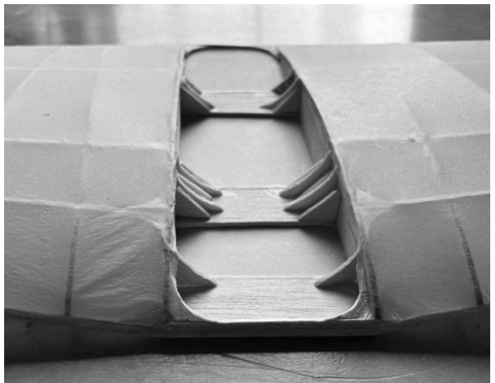
"H" tongues on Dave's 24" Lockheed P80. Tongues extend into the fuselage interior and are glue into place between two well-reinforced formers.
