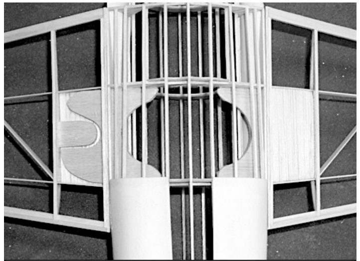
Left side shows the "H" tongue, in place in the wing box, which is built up between the spars and two ribs. Note the additional tab at the left side of the wing box, which is glued to the top and bottom of the box for reinforcement. On the right side, the box has been closed up.
