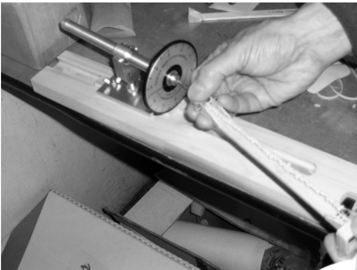
14. Hold the yoke and insert the peg in the rear notches of the loading stick. Remove the yoke.
